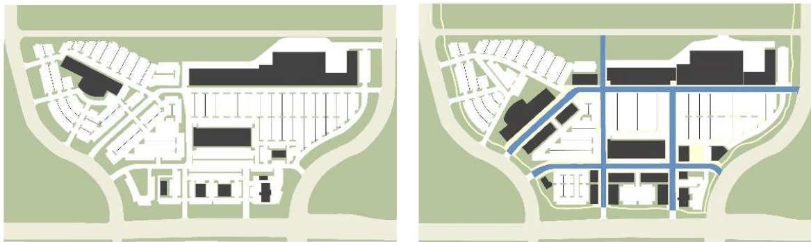
Figure 3-2 Private streetscapes. Private streetscapes shall be used to mimic public street networks and streetscapes for over-sized parcels and large scape development (17-3-1.B.2.d).
